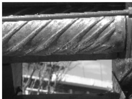
Fig. 3: Helical gear around the roller
